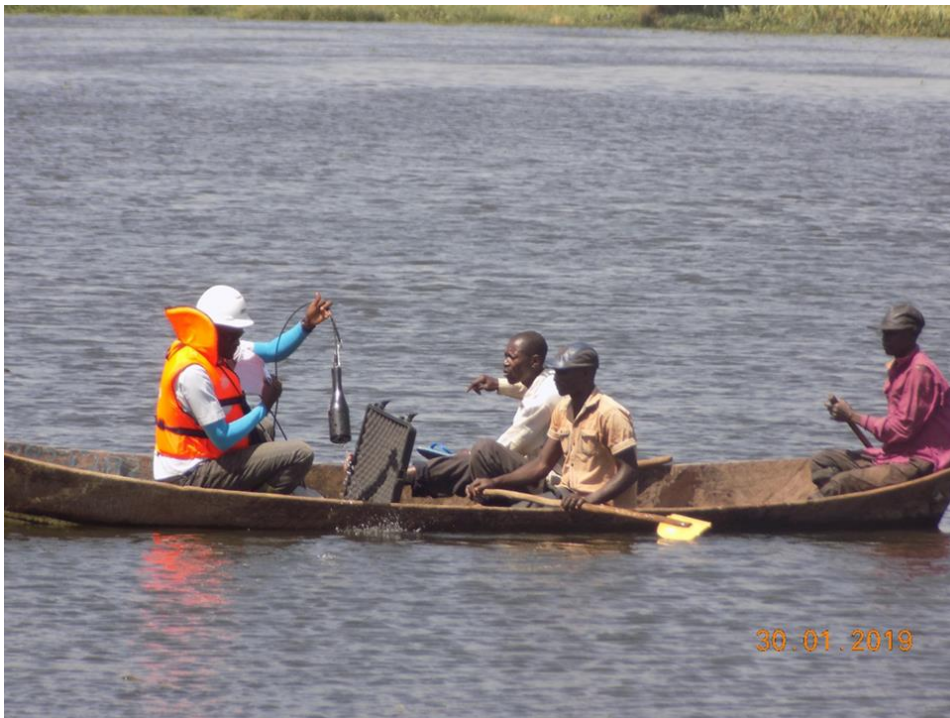
ESIA- measurements for Physio-Chemical Analyses using Horiba Water Quality Monitor
